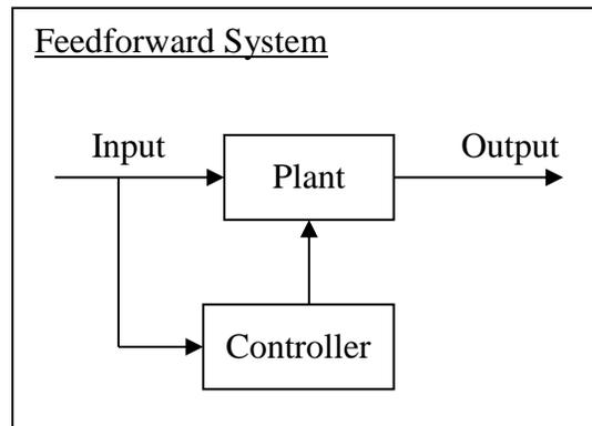
If the behaviour of a plant is *linear*, that is, if it can be described using a *linear algebraic* or a *linear differential* equation, then the plant can be described using a *transfer function*, indicated by  $G(s)$  in the diagram below. The purpose of a transfer function is to provide an *accurate quantitative representation* of the output of the plant given its input. Transfer functions associated with linear differential equations can be found using *Laplace transforms*.
