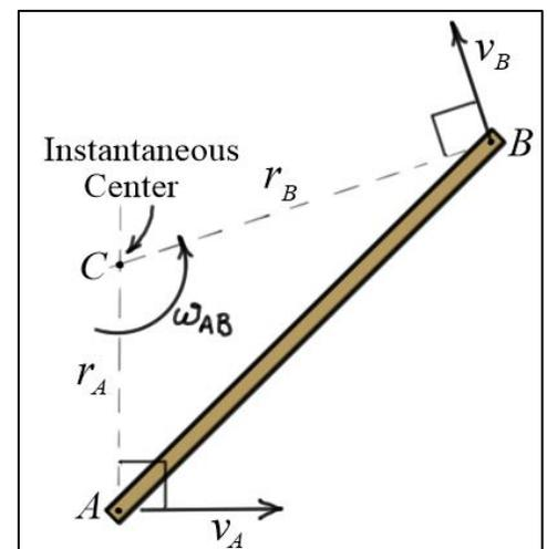
The velocities of the two points are  $v_A = r_A \omega_{AB}$  and  $v_B = r_B \omega_{AB}$ . The *instantaneous center*  $C$  will be in *different locations* from *one instant* to the *next*.
