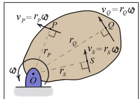
For example, the magnitude of the velocity of point  $P$  can be written as  $v_P = r_P \omega$ . The direction of the velocity is perpendicular to the line connecting  $O$  and  $P$ .
