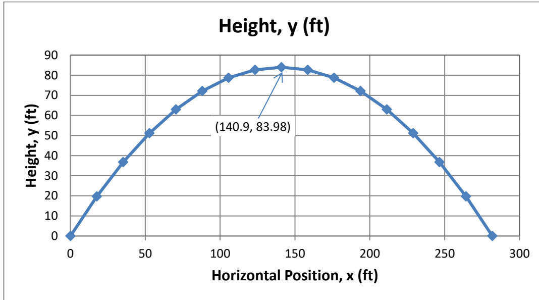
Figure 1. Height of Golf Ball as a Function of Distance, x
