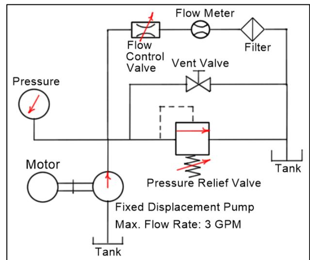
Fig. 3: A circuit to control the flow rate of hydraulic fluid.
