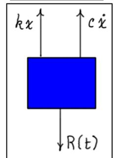
Here, the variable  $x$  is measured from the *equilibrium position*. Note that *static forces* are *not present* in this equation.
