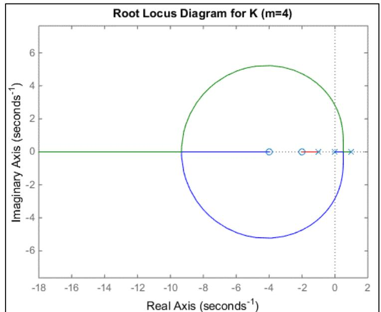
The **three branches** of the diagram are shown in green, blue, and red. Note, however, that MATLAB **does not show** the **direction** of the **movement** of the poles as  $K$  increases. It is **understood** the movement is **from the poles** of  $P(s)$  **to the zeros** of  $P(s)$ . In this case, there are
