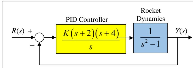
The **characteristic equation** of the closed-loop system is  $1+GH(s)=0$  or  $1+KP(s)=0$ . Substituting the transfer functions from the block diagram into the characteristic equation gives
